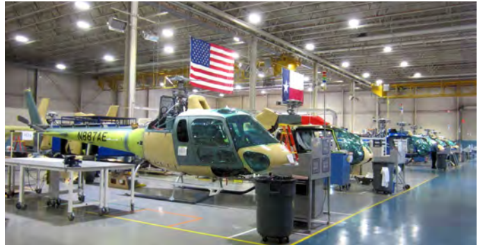
Airbus H125 (previously the Eurocopter AS350B3e) AStars and H130 (EC130) Ecostars sit in assembly at the Grand Prairie plant in 2014. (AHS photo)
