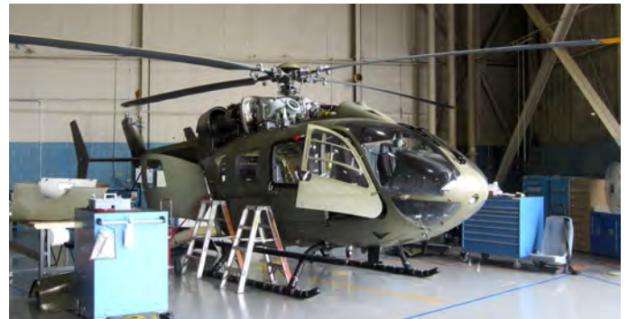
The Army bought the EC145 as the UH-72 Lakota, which is built in Columbus, Mississippi. (Note the contrast to the Dallas Cowboy's newer H145, which has the Fenestron tail rotor.) This aircraft, seen in Grand Prairie in 2014, was a company demonstrator. (AHS photo)
